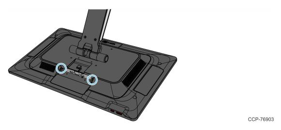
5. Rotate the Back Cover away from the Display and unhook the Back Cover Tabs.
