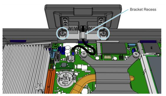
8. Connect the APA Graphical Display Cable to the Motherboard.
