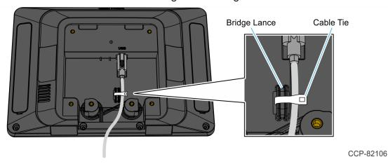
10. Install the XL10 Customer Display on the Bracket (4 screws). Ensure the Cable is routed through the gap in the Bracket as shown.
