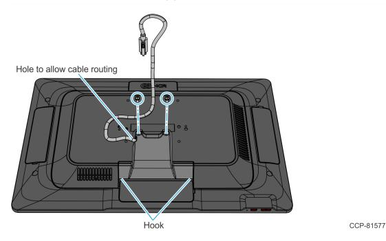
5. Partially install two (2) screws on the back of the CX7 Display in the location shown.
