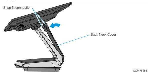
2. Install the Base Rear Foot (2 screws). Ensure the Neck Cover is captured under the Base Rear Foot.
