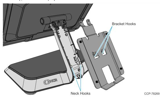
b. Secure the Bracket to the Neck with two (2) screws. Ensure no cables are pinched.
