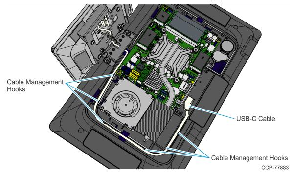
Confidential and proprietary information of NCR Voyix. Use and disclose solely pursuant to company instructions. 12. Secure the Cable under the Cable Management Hooks of the Bracket.
