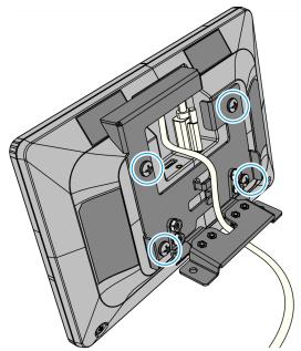
10. Install the Customer Display and Bracket assembly on the CX7 Display (2 screws).
