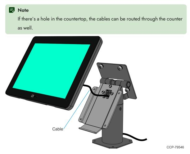
5. Install the Display on the Customer Display Bracket (4 screws).
