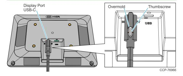
4. Route the XL7 Display Cable through the Customer Display Bracket and down the Pole.
