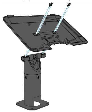
8. Install the Back Cover and Pole Assembly on the Display.
