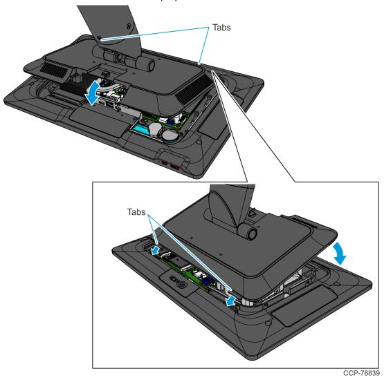
b. Secure the Back Cover with two (2) captive screws.
