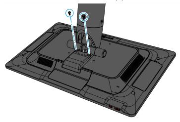
12. Install the Pole on the countertop using four (4) M4 wood screws (one on each corner).
