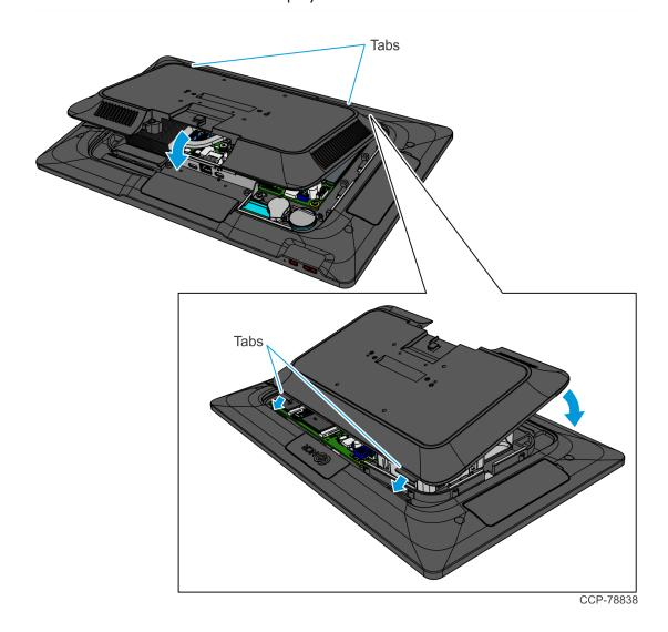
b. Secure the Back Cover with two (2) captive screws.
