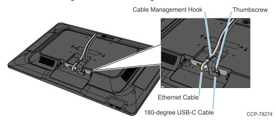
9. Route the Cables through the Bracket and down the Pole.
