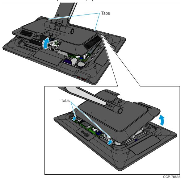
6. Remove the four (4) screws securing the Display Back Cover to the hinge of the Base.
