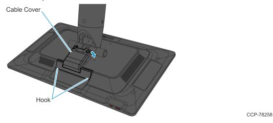
b. Secure the Cable Cover with two (2) screws.
