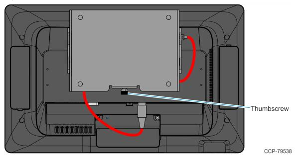
7. Connect the Power Cord to the Power Supply.
