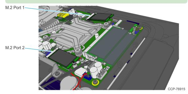
7. Secure the M.2 SSD to the Motherboard with a screw.
