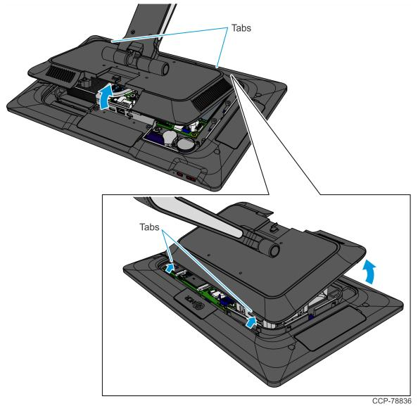
6. Insert a flat screw driver in the slot of Port C to unsnap the Plate from the display housing.
