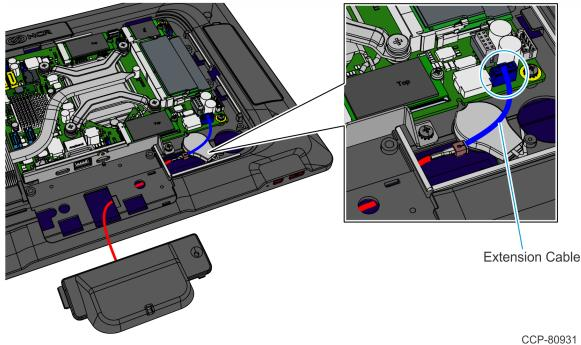
10. Hook the External Speaker into the display housing and snap into place.
