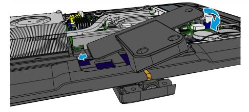
10. Secure the Rear Housing with three (3) screws.
