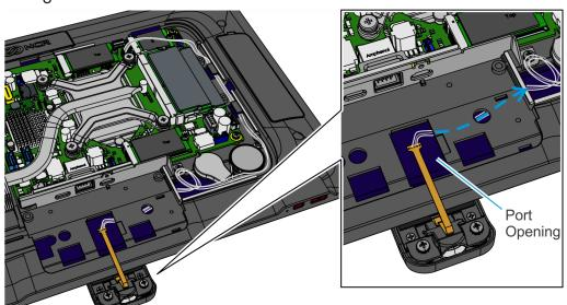
8. Route and secure the Cable under the Cable Management Hooks as shown, then connect the Cable to the Motherboard. Place excess cable in the area shown.
