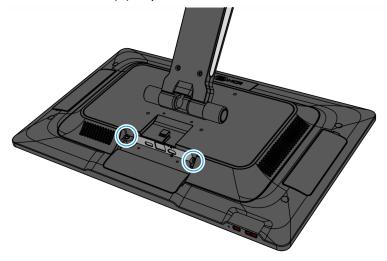
5. Rotate the Back Cover away from the Display and unhook the Back Cover Tabs.
