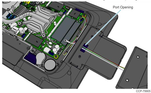
10. Route and secure the Bill Validator Cable under the Cable Management Hooks as shown.
