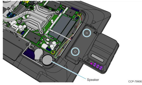
13. Secure the Ground Cable under the corner Motherboard Screw.
