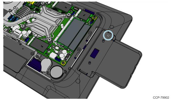
9. Route the Bill Validator Cable and the Ground Cable through the Port opening.
