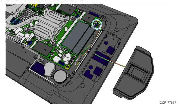
Hook the Biometrics into the display housing and snap into place.
