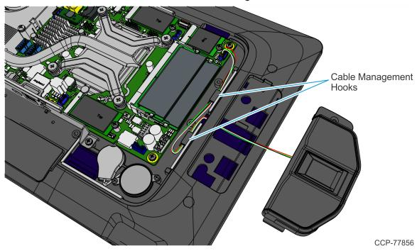
8. Connect the Cable to the Motherboard.
