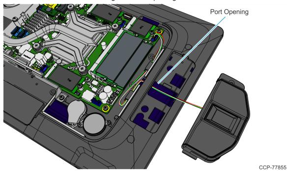
7. Route and secure the Cable under the Cable Management Hooks as shown.
