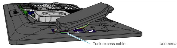
10. Hook the MSR into the display housing and snap into place.
