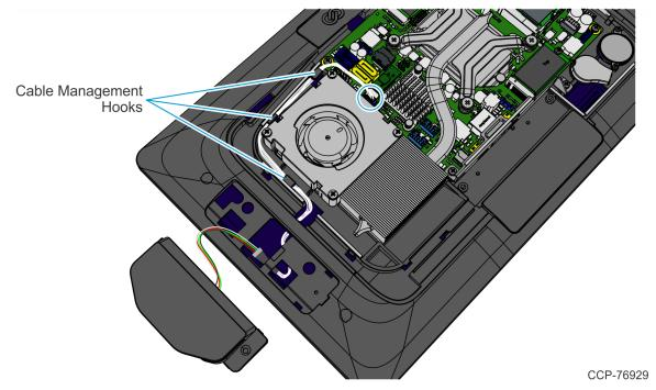
9. Tuck the excess Cable under the display housing.
