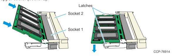
3. Press the Memory Module down until it latches in position. Ensure the latches are completely engaged.
