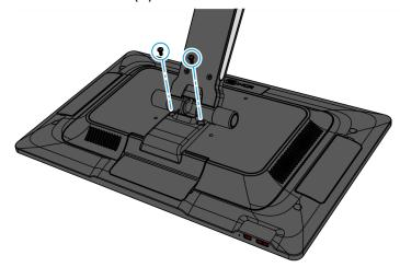
b. Rotate and unhook the Cable Cover from the Back Cover.
