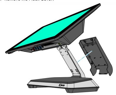
4. Snap the Back Neck Cover onto the neck. The Cover has a simple snap fit connection at the top.
