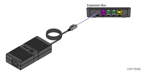
2. Connect the Power Supply Cable to the Expansion Box.
