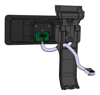
12. Secure the neck mount to the back of the 2x20 display using screws (2).
