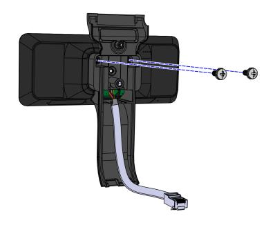
12. Secure the neck mount to the back of the 2x20 display using screws (2).
