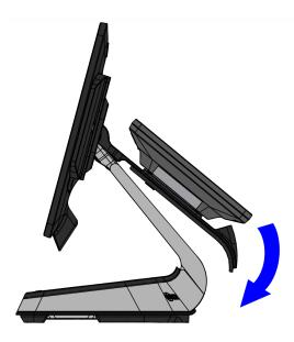
15. Secure the neck mount and XL7 display assembly on the neck of the PX10 terminal with a screw.
