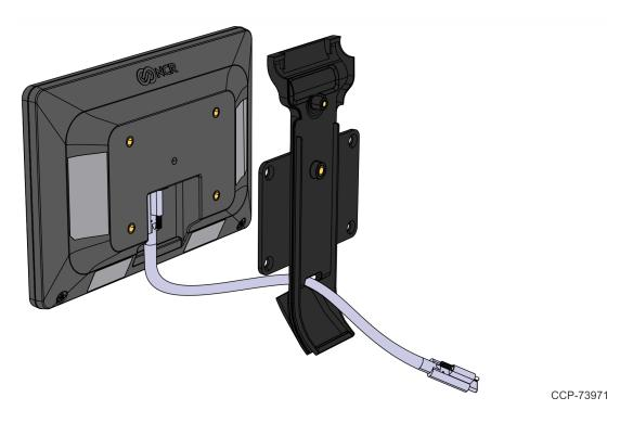
12. Install the neck mount to the back of the XL7 display using screws (4).
