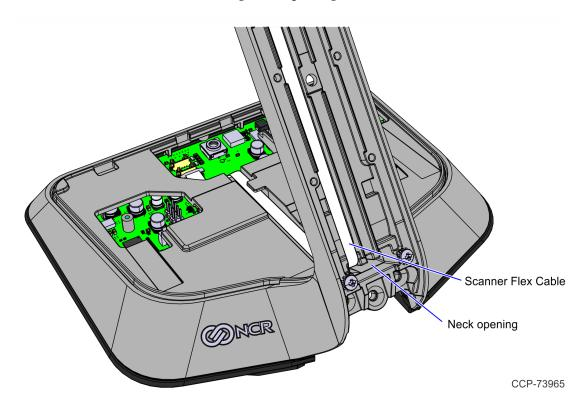
12. Route the scanner flex cable through the routing slot and connect the flex cable to the Motherboard with the blue side facing the front of the terminal.Scanner Flex Cable
