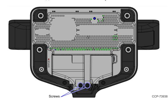
5. Remove the screws (2) that secure the Rear Base Cap to the Neck.
