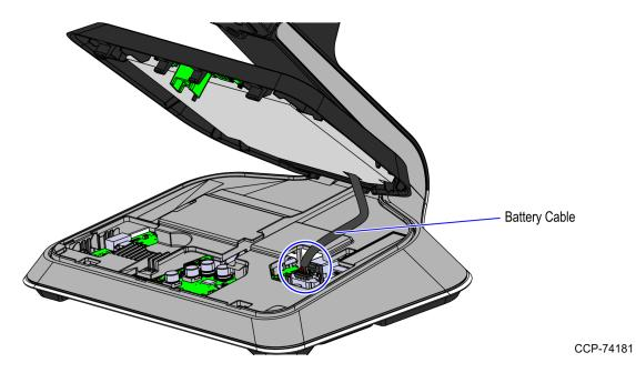
10. For versions with battery, disconnect the battery cable from the Motherboard.
