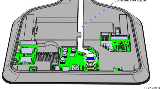
13. Position the rear scanner on the neck and pivot down.
