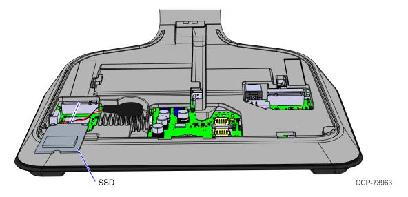
7. Secure the SSD in place using a screw (1).
