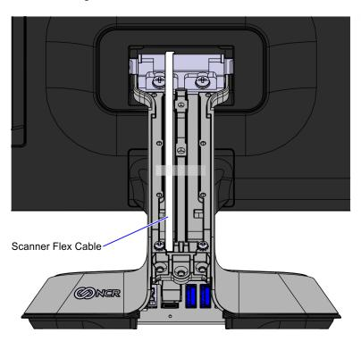
17. Insert the scanner cable through the opening at the bottom of the neck.
