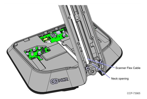
18. Route the scanner flex cable through the routing slot and connect the flex cable to the Motherboard with the blue side facing out.
