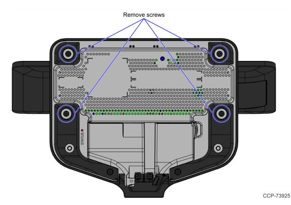
2. Using the screws included in the kit, mount a magnet into each of the four previous screw locations.
