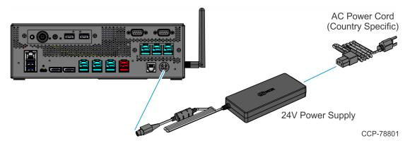
4. Connect the AC Power Cord to the Power Supply, then to an AC outlet.
