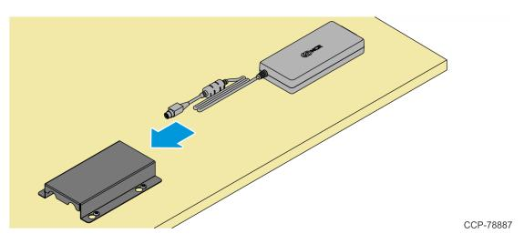
3. Connect the Power Supply Cable to the Power In connector on the terminal.
