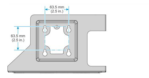
2. Insert the CX8 into the Mounting Bracket. The CX8 can be inserted in two (2) ways:
