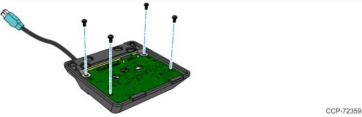
d. Install the Serial Expansion Module to the Stand (3 screws).
