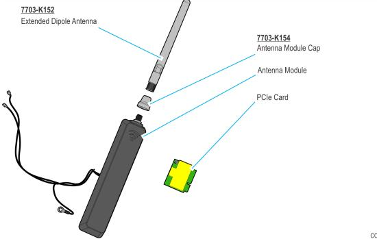
These kits provide the wireless network components for the RealPOS XR7 Plus POS.
