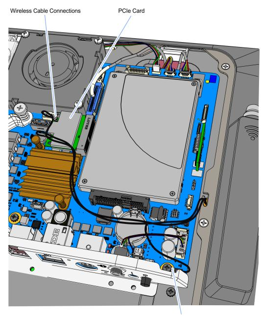
8. Install the PCIe Card on the Motherboard connector and secure it with a screw.
