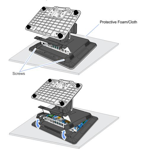
3. Remove the Display Collar (9 screws).
