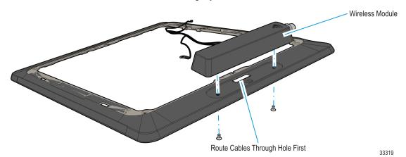
6. Route the Wireless Cable through the Cable Guide on the Display Collar.
