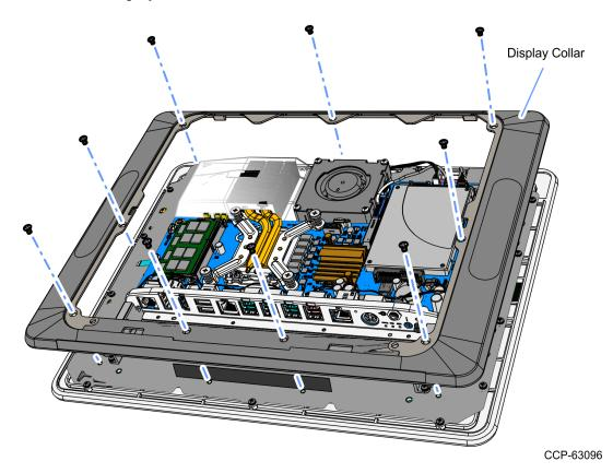
4. Remove the Blank Plate (left side of terminal, right side is for MSR) from the Display Collar. The plate is connected to the Display Collar with a strong adhesive. Use care when removing it to not damage the Display Collar.
