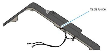
7. Install the Display Collar onto the terminal.
