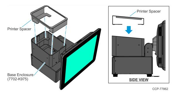
3. Place the Printer in the Printer Spacer recess.
