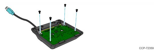
c. Remove the Serial Expansion Board from the Serial Expansion Housing.
