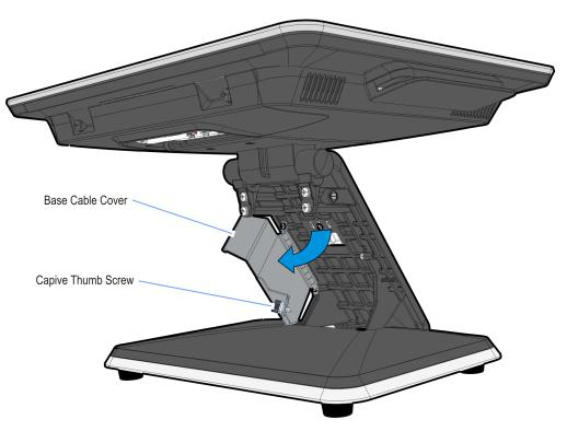
6. Loosen the captive thumb screw on the Base Cable Cover and pivot it open.
