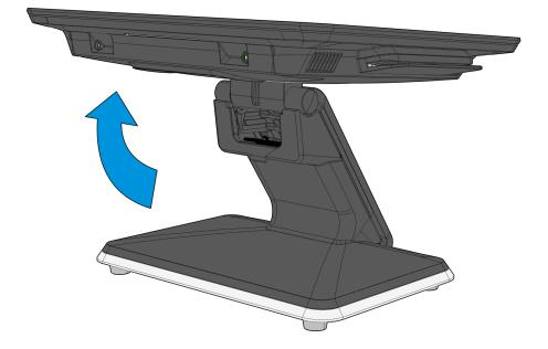
4. Pivot the POS display to a horizontal position.
