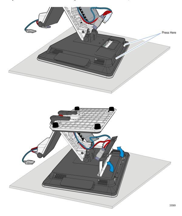
10. Open the Terminal Cable Cover (press in at the indentations).
