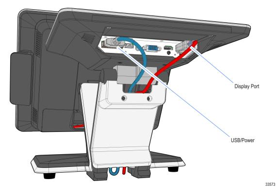
17. Connect the USB+12V Cable and Display Port Cable to the Customer Display.
