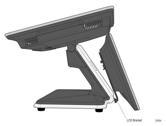
b. Pivot the assembly into position on the POS Stand and secure it from inside the stand with screws (2).
