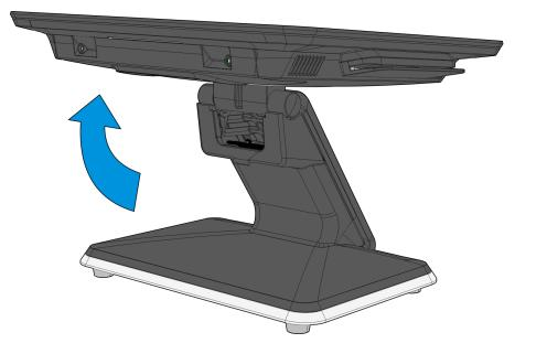
2. Remove the Upper Stand Cover by pivoting it away from the stand. The cover has a simple snap fit connection at the top.
