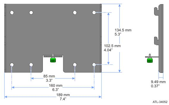
2. Install the 497-0509698 Power Supply Wall Mount Bracket onto the back of the terminal with the supplied screws (4).
