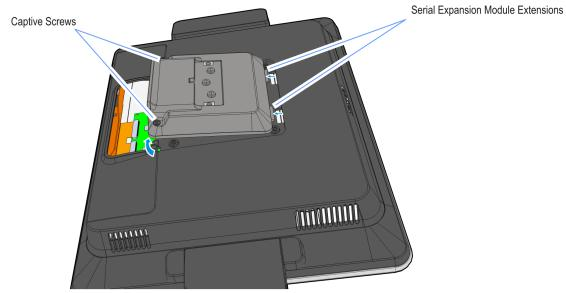
3. Install the Wall Mount Bracket (with the thumbscrew facing up) onto the Serial Expansion Module with the supplied screws (3).
