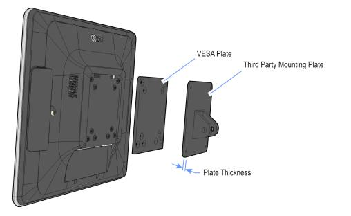
**Note:** For 15" 5968/5985 RealPOS X-Series Displays, use the 75 mm or 100 mm pattern on the VESA Plate. For 10.4" 5968/5985 RealPOS X-Series Displays, use the 75 mm pattern.
