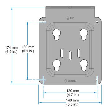
2. Install the Wall Mount Bracket (with the thumb screw facing up) onto the back of the terminal with the supplied screws (4). Use the appropriate screws for the terminal.
