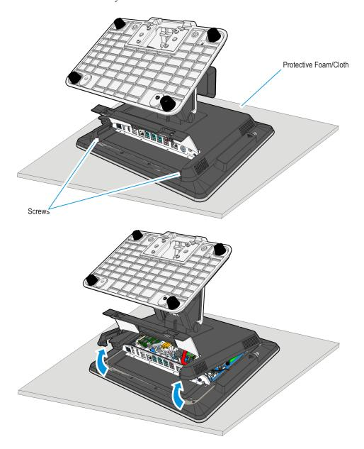
3. Remove the Display Collar (9 screws).
