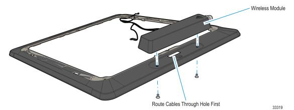
6. Route the Wireless Cable through the Cable Guide on the Display Collar.
