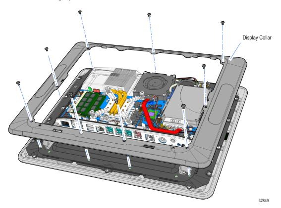
4. Remove the Blank Plate (left side of terminal, right side is for MSR) from the Display Collar. The plate is connected to the Display Collar with a strong adhesive. Use care when removing it to not damage the Display Collar.
