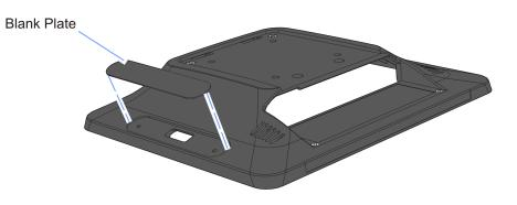
5. Install the Biometrics Reader on the Rear Cover (2 screws).
