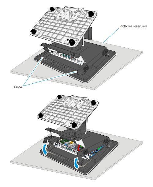
3. Remove the Display Collar (9 screws).
