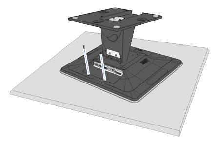
2. Pivot the Stand and Rear Cover assembly as shown to remove it.
