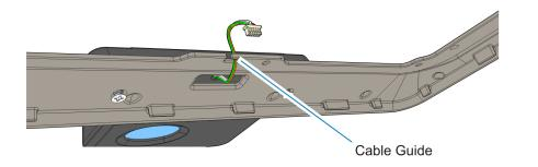
7. Install the Display Collar onto the terminal (7 screws).
