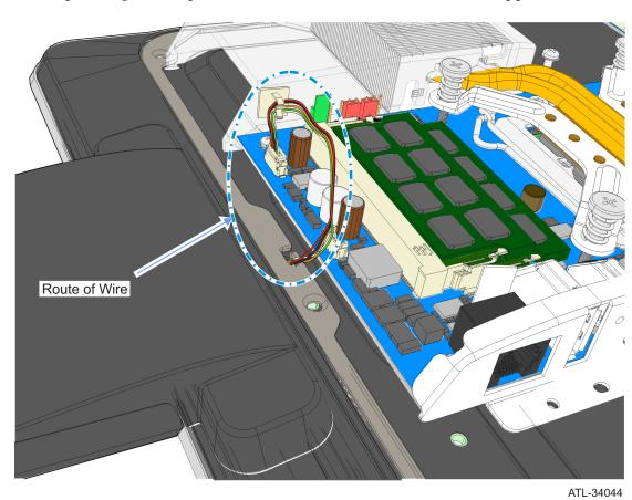
**Note:** When installing the Biometrics Reader on the right side (Port A), route the cable up through the clip and connect the Biometrics Cable to the upper connector.
