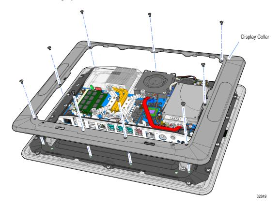
4. Remove the desired Blank Plate from the Display Collar. The plate is connected to the Display Collar with a strong adhesive. Use care when removing it to not damage the Display Collar.
