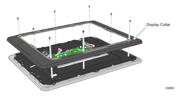
4. Remove the Blank Plate from the Display Collar. The plate is connected to the Display Collar with a strong adhesive. Use care when removing it to not damage the Display Collar.
