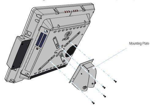
2. Extend the Mounting Plate Latches outward as shown and install the 7404 onto the Baseplate. The two studs on the Mounting Plate are inserted into the two slots on the Baseplate. The Mounting Plate Latches are spring loaded and lock into the holes in the side of the Baseplate.
