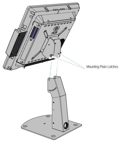
3. Adjust the angle of the 7404 as desired. The screen can be adjusted from 0 degrees (vertical) – 54 degrees (from vertical), in 9 degree increments.
