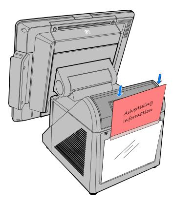
4. Insert the top two tabs into the top slots in the cabinet by flexing the Signage Insert.
