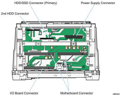
4. Install the Secondary HDD in the upper HDD slot.
