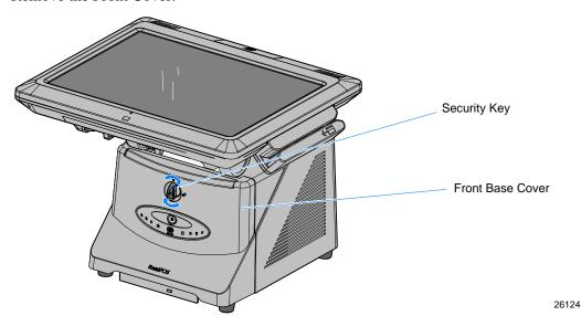
c. Pivot the top of the Front Base Cover toward the front of the unit and remove it from the terminal.
