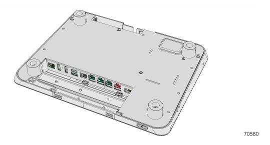
2. To open the I/O Cover, press on the ribs on both sides and then pivot the cover.
