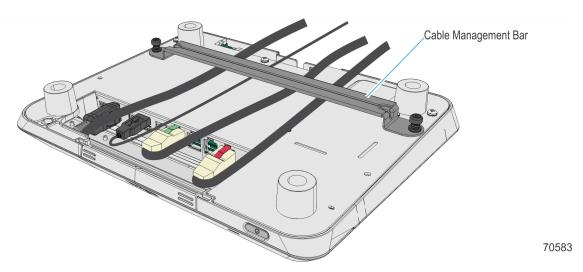
6. Tighten the thumbscrews (2) to secure the cables.
