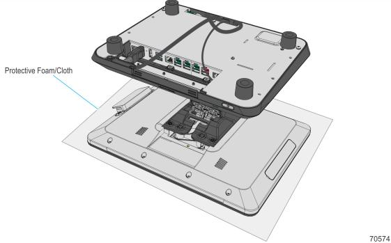
2. To open the I/O Cover, press on the ribs on both sides and then pivot the cover.
