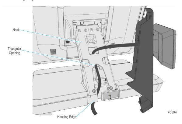
7. Route the cable through the neck, into the triangular opening, and then under the housing edge.
