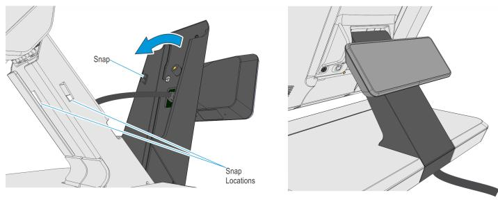
9. Rotate the assembly to fit the neck. Snap the assembly into place.
