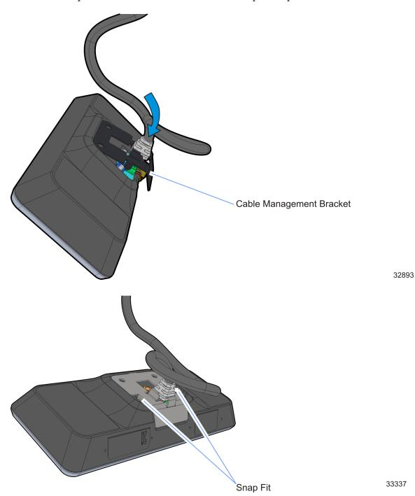
4. Insert the tab in the edge of the Cable Management Bracket in the slot in the Rear Cover and pivot the bracket as shown until it snaps into position.
