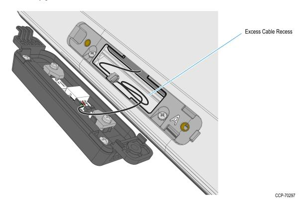
4. Hook the Encrypted MSR to the Back Housing and snap into place.
