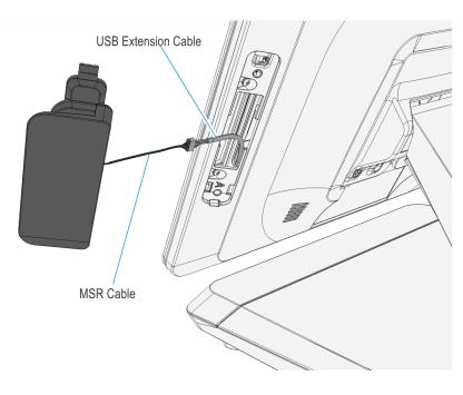
3. Gently push the excess cables into Port A recess.
