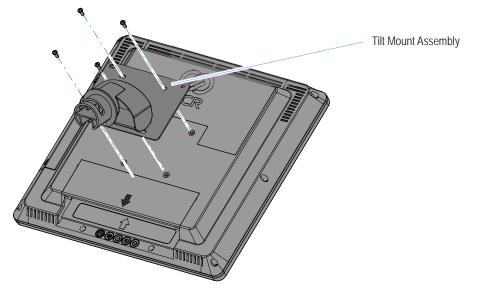
2. Install the Customer Display Base (7610-K452) on the back of the 7610 *Table Top Stand* (7610-K320). Secure it with screws (2).
