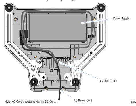
8. Replace the Power Supply Cover (4 captive screws). Make sure the screw holes are not obstructed by the power cords before installing the cover.
