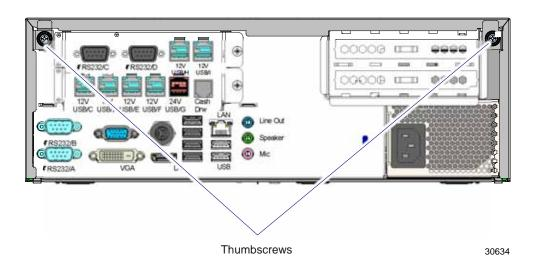
4. Slide the cover toward the rear of the terminal to remove it.
