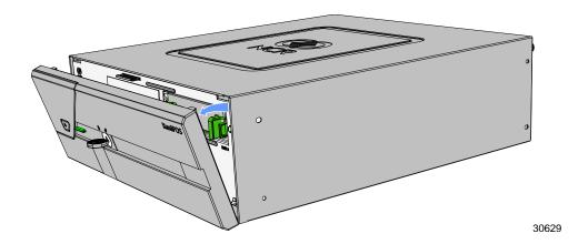
3. Loosen the thumbscrews (2) that secure the Top Cover.
